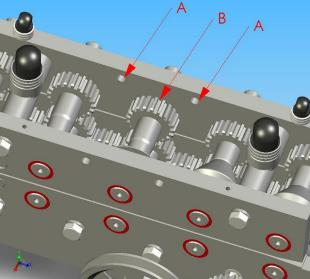
6. Secure the RAMS 2008 Power Flanger using the 3/8-16 x 1-1/4" hex head cap screws and lock washers described in item #2. Use mounting holes (A). (see picture on previous page)
