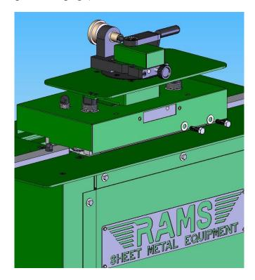
7. Place the side access panels back on the top cover. Below is a view of completed installation.
