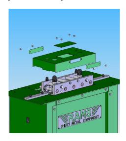
3. Remove the supplied 3/8-16 x 1-1/4" hex bolts and 3/8" lock washers. Make sure to keep these components, as they will be needed when fastening the power flanger.
