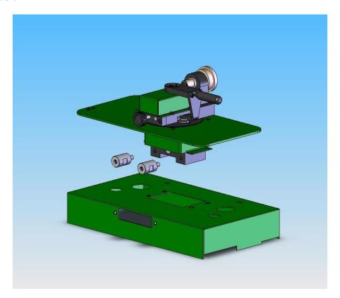
5. Set the flanger attachment over the forming head so that the combination bevel and spur gear meshes with the Pittsburgh Lock roll (B). Use mounting holes (A).
